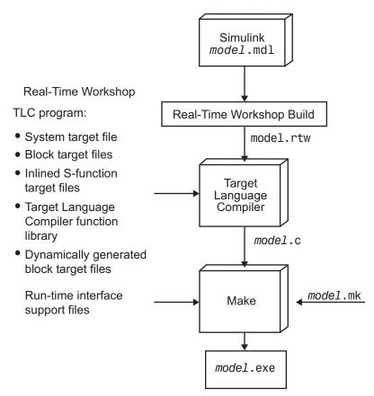
The process of generating source code from Simulink models using Real-Time Workshop is shown in the following diagram.
